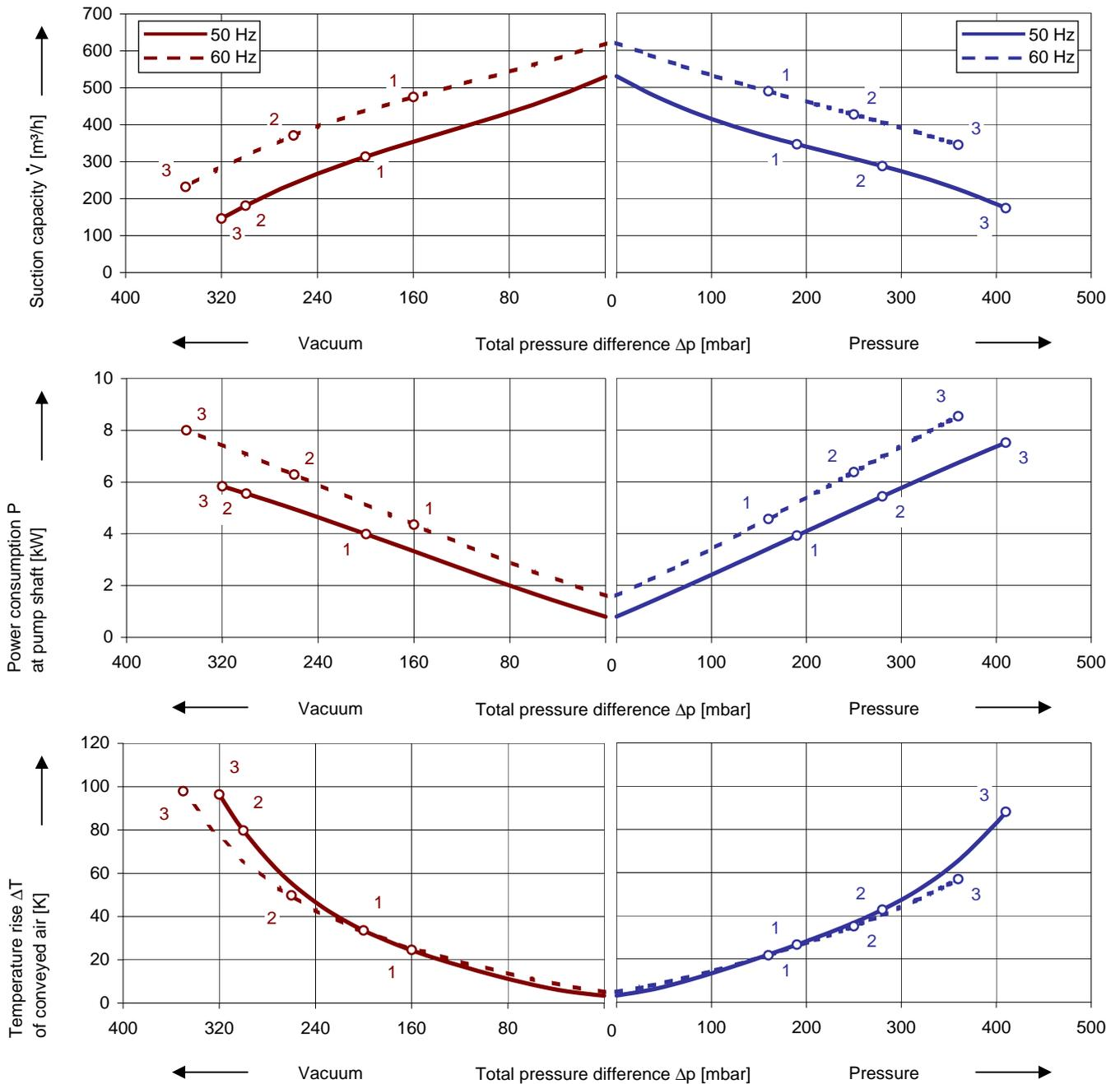
The performance curves are based on air at a temperature of 15 °C and an atmospheric pressure of 1013 mbar with a tolerance of  $\pm 10\%$ . The total pressure differences are valid for suction and ambient temperature up to 25 °C. For other conditions please get in touch with us.
