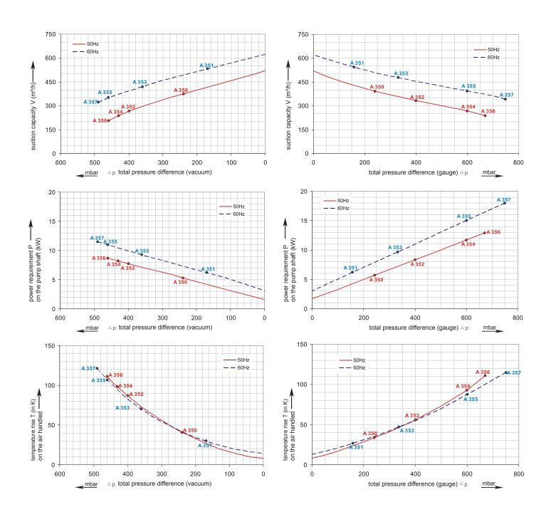
The performance curves are based on air at a temperature of 15  $^{\circ}$ C and an atmospheric pressure of 1013 mbar with a tolerance of +/- 10  $^{\circ}$ C. The total pressure differences are valid for suction and ambient temperatures
